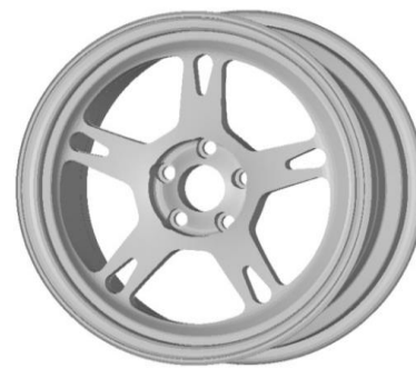
Figure 20: The optimized design after topology optimization
